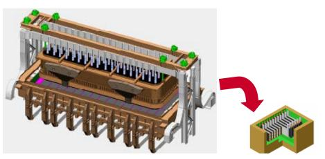
200 kA cell with carbon anodes 200 kA cell with vertical inert anodes
